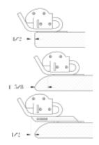
This diagram shows extended (on right) and raised (on bottom) modification options available. Due to bending concerns, Forespar® offers a 4" maximum extension. The upper far right image is the standard davit head, and the rest are
