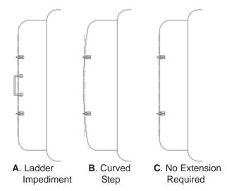
This diagram shows a swim step with a rounded trailing edge which requires the davit head mounting plate be moved forward to attach to a flat surface. Again, this condition would require an aft extension modification to move the yoke bearing point in the davit head so there would be a minimum 1/2" to the aft of the swim step edge.
